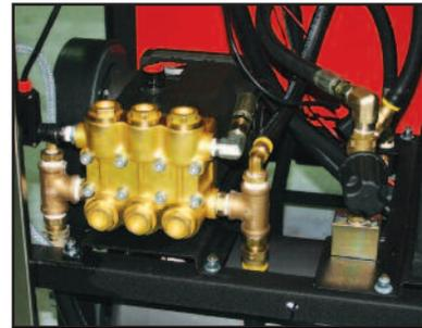
**Large frame Hotsy belt-drive pump** features NESTechnology with U-Seals for 3 times longer pump life.
