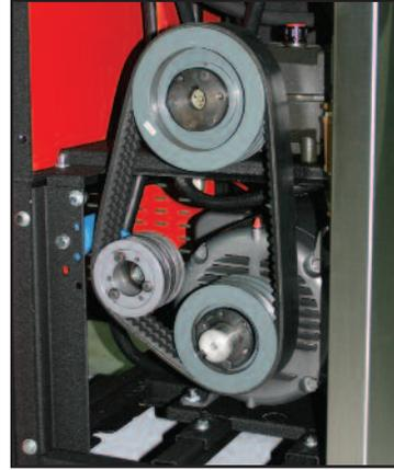
**Vertical banded belt** provides extended life and reduced maintenance costs by eliminating multiple belts that stretch at different rates. New belt tensioner provides constant tension and makes servicing and maintenance of the belt a breeze.
