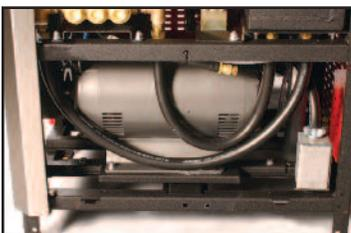
Motor is mounted to **slide out rails** for easy removal
