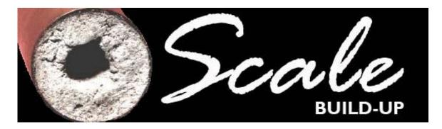
Lime and scale build-up in a pressure washer coil is caused by hard water leaving silicates, sulfates, and similar materials that will interfere with proper coil operation. This buildup of debris will result in corrosion, reduced water pressure and less water volume. Preventing scale from building up or "descaling" will increase equipment efficiency, prolong the life of the coil and ultimately save money.
