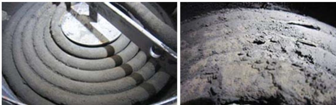
Soot build-up on the heat exchange coil is a symptom of an ill-maintained burner. Soot causes a variety of problems including difficulties with draft, efficiency, and carbon monoxide. Soot plugs the coil and reduces the airflow which in turn, reduces the pressure washer's efficiency and overall equipment life. As soot builds up on the burner coil, fuel consumption and costs increase.
