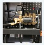
Large frame Hotsy beltdrive pump features NESTechnology with U-Seals for 3 times longer pump life. The pump also has an oil drain, allowing for easy oil changes.
